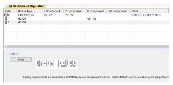
At this time we can use FROM instruction to read the module's temperature value, because the module is in the second module position of hardware configuration, in the FROM instruction, we set Slot = 2, hex 10H, that is, the decimal 16, so the program as follows:
