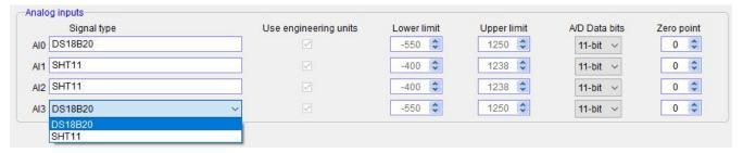
In addition, we can see that when choosing to measure the temperature and humidity, the analog input register does not appear two consecutive addresses, such as the above channel 2 and 3 are connected to temperature & humidity sensor SHT11, but only one Al1 and Al2 indicates the measured temperature value. So how to read the humidity value?
