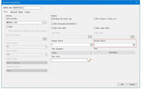
So that when the PLC read Al0 value, Al0=123, that is the actual value of  $12.3^{\circ}$ C, there is no need to have data processing in PLC and configuration, only set the 1 decimal places on the numerical display primitive, then it will be automatically reduced by 10 times, displaying value of 12.3, that is the actual value of 12.3 $^{\circ}$ C.
