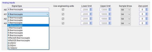
In this way, after configuration, as long as connect the K-type thermocouple to channel 1, then directly read Al0 register value, Al0
