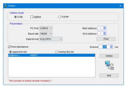
If there is only one machine connected with 485 line, then check "stand-alone search"; if there are more than one, then remove the button of "stand-alone search", and set the start address and end address, so that all the machines connected with 485 line can be found and achieve parameter configuration.
