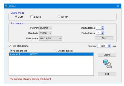
Click "exit", or "×" to exit. In the absence of sensors, the default parameters of the module are shown below:
