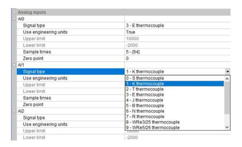
After setting, select the "Download parameter" to download the parameter into the module.
