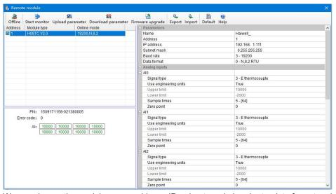
We can change the module name, address, IP, subnet mask, baud rate, data format and other communication parameters in the communication parameter area.
