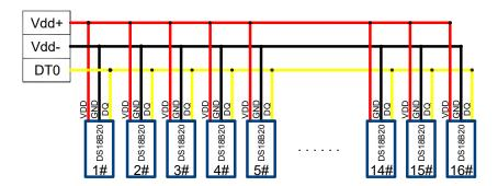
After the 16 sensors of channel 1 accessed, channel 2 is accessed in the same way, when accessed, we follow the way from near to far or from far to near. After finishing the access of all sensors, we have to save the configuration parameters of H32DT module, this step is very important! (The back will introduce the application occasions). The specific operation is as follows, in the menu bar of remote module tool has an export function, we click export:
