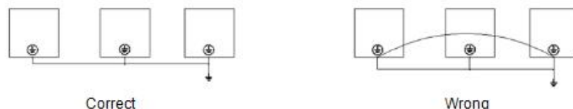
Figure 3-8 Grounding Wire Connection Sketch Map
